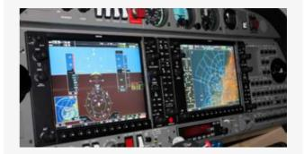
State of the art Diamond Aircraft DA40 and DA42 fleet fitted with the latest Garmin G1000 avionics.
